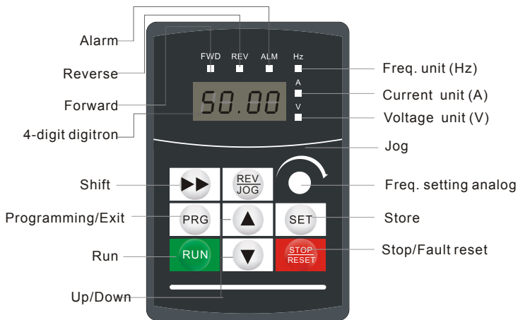
Diagram 4-2 Keyboard of CV3100 inverter
